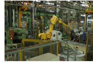
Gravity die casting cell
